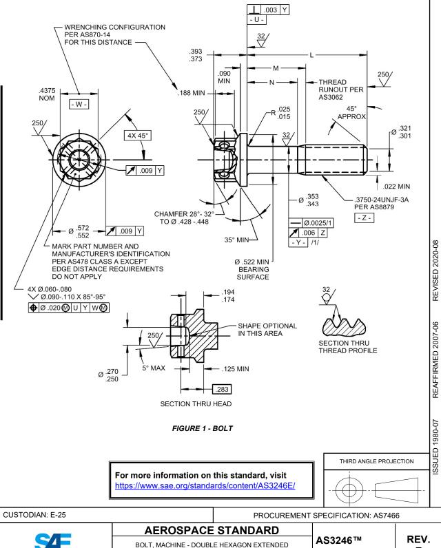
WASHER HEAD, DRILLED, PD SHANK, NICKEL ALLOY, UNS N07718, 185 KSI MIN, .3750-24 UNJF-3A
